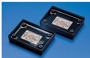
Electronic components potted with silicone gel
