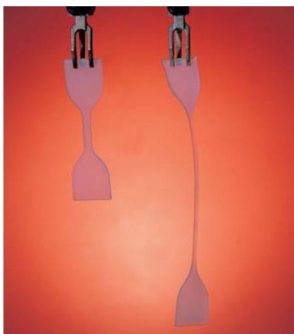
Crosslinked polyethylene: heat resistance test
